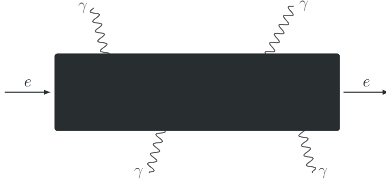
(a) Electron passing through a layer of material undergo multiple scatterings, which lead to production of photons.
