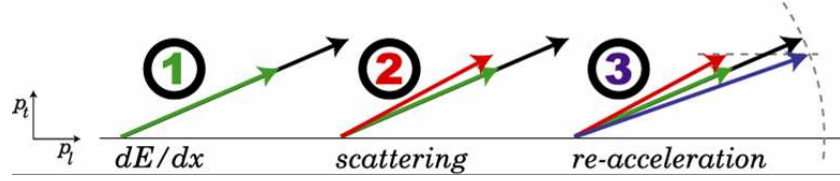
Figure 8.1: Fundamental principle of the ionization cooling: reduction of the transverse momentum after passage through absorber and RF cavity.
